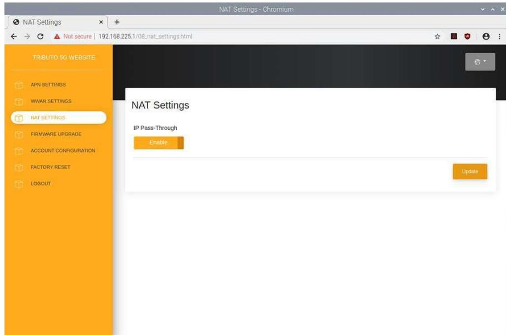
Dongle will reboot after enabled IP pass-through.
